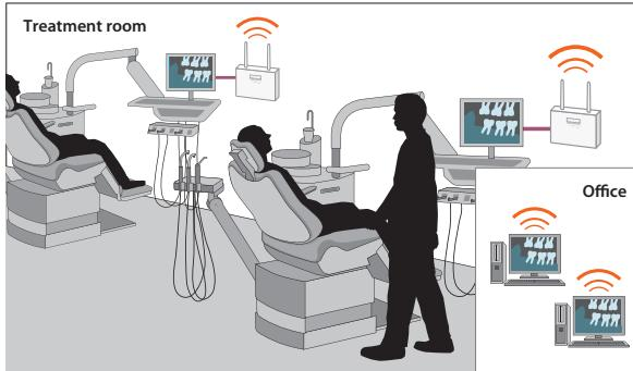
The monitor next to the treatment chain is wirelessly connected to the PC in the office, so that patient files and X-rays can be called up there. This means that there is no need to set up a PC next to each treatment chair, which has a positive effect on the room design.
